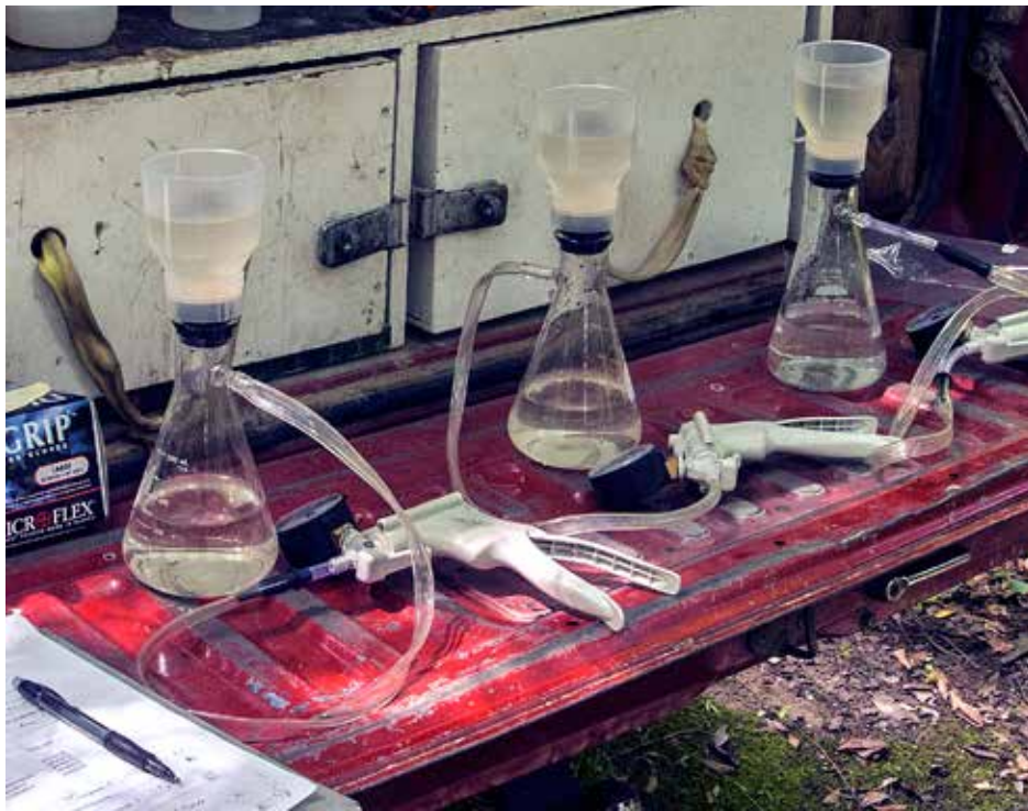
In the field, water filtration using hand operated vacuum pumps. PHOTO CREDIT: JIM GODWIN
