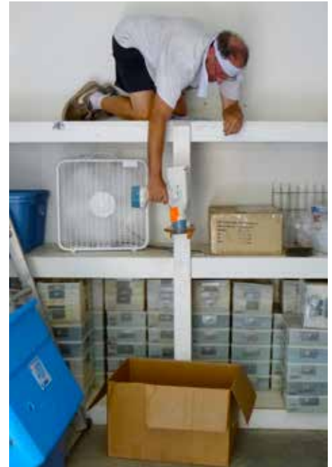
The Nomad, a portable, dental x-ray machine, was on loan from the Aribex Company. The turtle is in the container on the floor. There's a cheap laser pointer taped to the machine for aiming purposes. An exposure time of 1 to 3 seconds produced excellent films.
